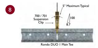
■ INSTALLING THE MAIN TEE INTO SUSPENSION CLIPS
