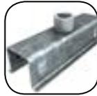
The U Clip™ is simply snapped into the underside of the TCR and then the threaded rod is screwed into the clip, using either 122 (threaded one end) or 123 (threaded both ends) Suspension Rods. The standard 121 Rod can be accommodated by joining it to the threaded rods with the 254 Joiner (also known as the 'Banana Clip').
