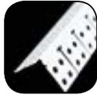
PEA90. One leg is pre-cut to allow the bead to be fixed around both outside and inside radiuses, providing a clean and engineered finish. Either spray adhesive or staples can secure this bead.
