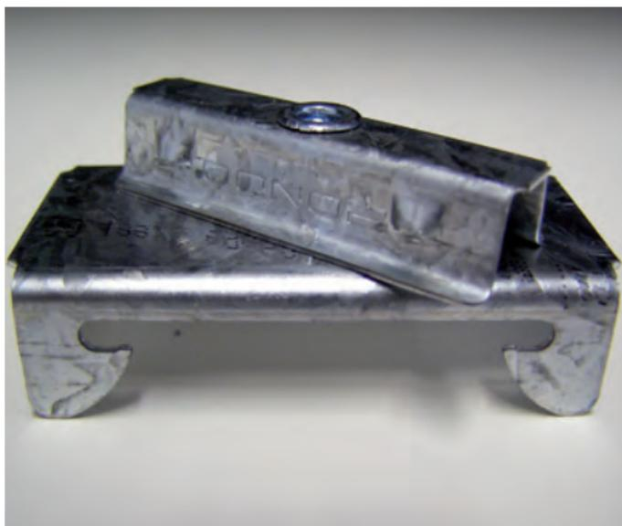
The new Rondo 238 Swivel Clip allows Rondo 129 or 308 Furring Channel to be attached to Top Cross Rail and be angled in any direction, offering Contractors flexibility during set out. >>
