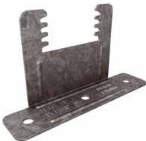
The new Rondo BG05K BETAFIL® Direct Fix Furring Channel Clip is a modified version of the Rondo BG05 BETAFIL® Double Membrane Insulation Clip. It suits rigid insulation board panels up to 50mm thickness, such as those supplied by Kingspan. >>
