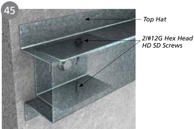
■ INSTALLATION OF TOP HAT TO CONCRETE
